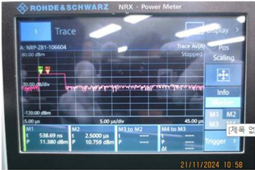
POUT ( Spike Leakage Power, Flat Leakage Power)
